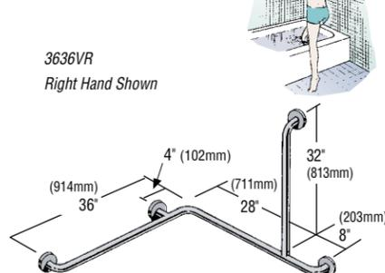
The 2040V and 3636V are excellent multi-purpose bars that provide a vertical arm and two horizontal supports for added stability. When entering tub, if the bather's right hand grips the vertical, specify right hand. If reverse, specify left.
