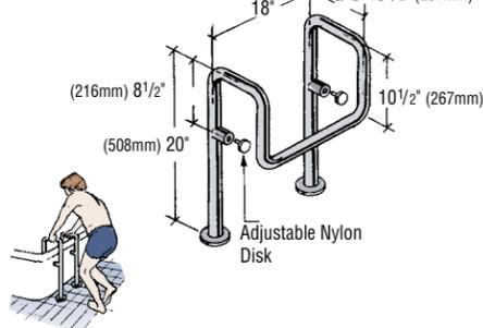
This bar provides a convenient grip for balance at tub entrance. The time-tested design combines floor mounting with a brace that adjusts against the tub for a snug fit. *Note:* Dimensions are for 16" (406mm) tub height. If different, please give tub height from floor.
