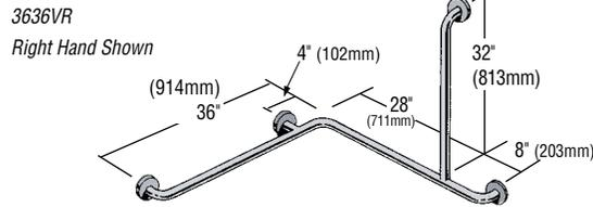
The 2424V and 3636V are multi-purpose bars that provide a vertical arm and two horizontal supports. When entering tub, if the bather's right hand grips the vertical, specify right hand. If reverse, specify left.
