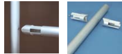
Tee Connection Use threaded rivet and stainless steel machine screw with lock washer for forming tees. Cross Assembly Where two 90° tees are mounted opposite each other to form a cross assembly, a stainless steel through bolt with lock nut may be used.
